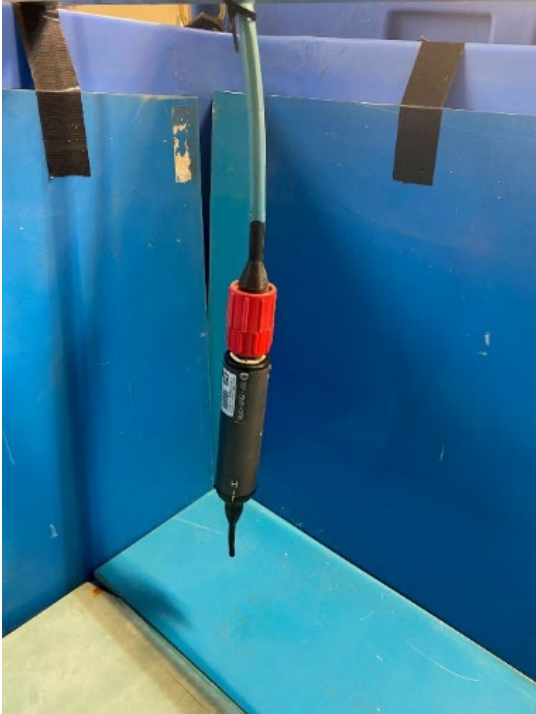
Figure 3. Raceway monitoring method 1: dipping a hydrophone into the raceway from the water surface.
